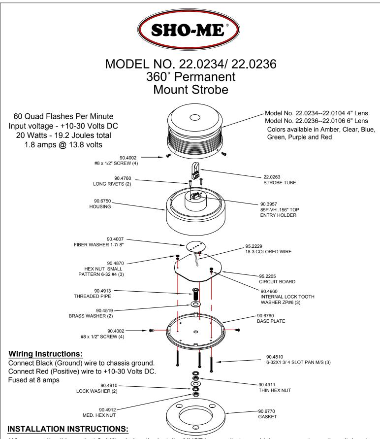
When mounting this product & drilling holes, the installer MUST be sure that no vehicle components or other vital parts could be damaged by the drilling process. Check both sides of the mounting surface before drilling begins. Also de-burr any holes and remove any metal shards or remnants. Install grommets into all wire passage holes.
