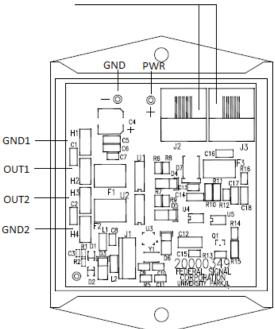
**3.** Connect the RS485 cable from any Federal Signal controller programmed to send relay commands, or the PA300-CN siren amplifier, to the two network terminals on the relay module.
