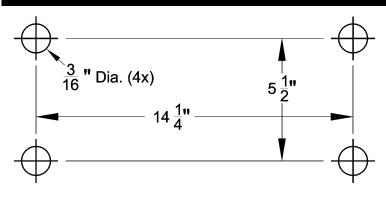
1. Mark the four mounting holes and drill a 3/16" hole each location.
