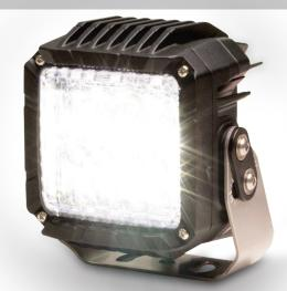
The CW2311 is a heavy-duty flood light that is designed to withstand tough jobs under extreme conditions. It delivers nearly 5,000 Lumens of intense light with its nine, ten-watt LEDs. The articulating worklight comes equipped with a stainless-steel bracket for easy installation. It features durable aluminum, heatsink housing along with a tough polycarbonate lens.
