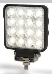
This deceptively powerful flood light emits over 2,000 lumens over 500 feet. It installs easily with a one-bolt, stainless steel bracket and features an adjustable head, aluminum heatsink housing and a tough polycarbonate lens. The light operates in the 12-24 VDC range and it is suitable for a wide variety of applications.
