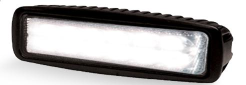
The CW2441 is a versatile LED worklight that can be mounted virtually anywhere on the vehicle or apparatus surface. Choose from flood or spot beam configurations to illuminate the scene or locate equipment. Although measuring just over six inches in length, the CW2441 is designed to resist weather and operate under extreme conditions with aluminum heatsink housing and a tough polycarbonate lens.
