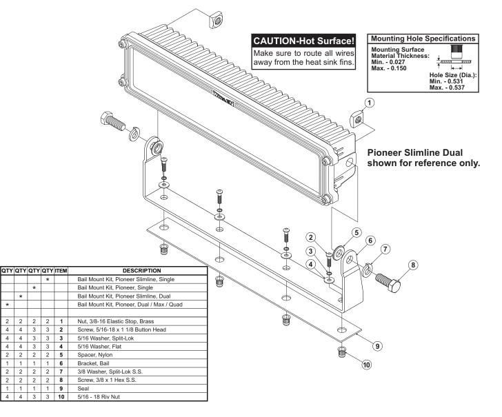
CAUTION: Mounting this product will require drilling. It is absolutely necessary to make sure that no other vehicle components could be damaged by this process. Check both sides of the mounting surface before starting. If damage is likely, select a different mounting location.
