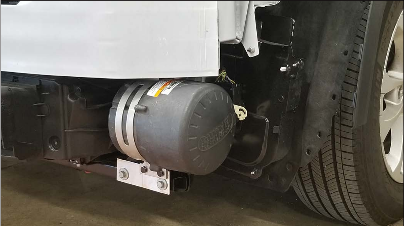
Figure 2 Installed Rumbler speaker (Prototype bracket shown)
